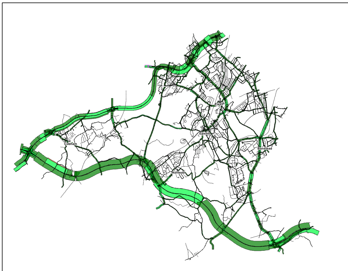
Figure 28 Local Model Link Flow versus Count Bandwidth for the PM Peak Hour (1700 – 1800) with all roads showing above and a close up of Epsom and Ewell below
