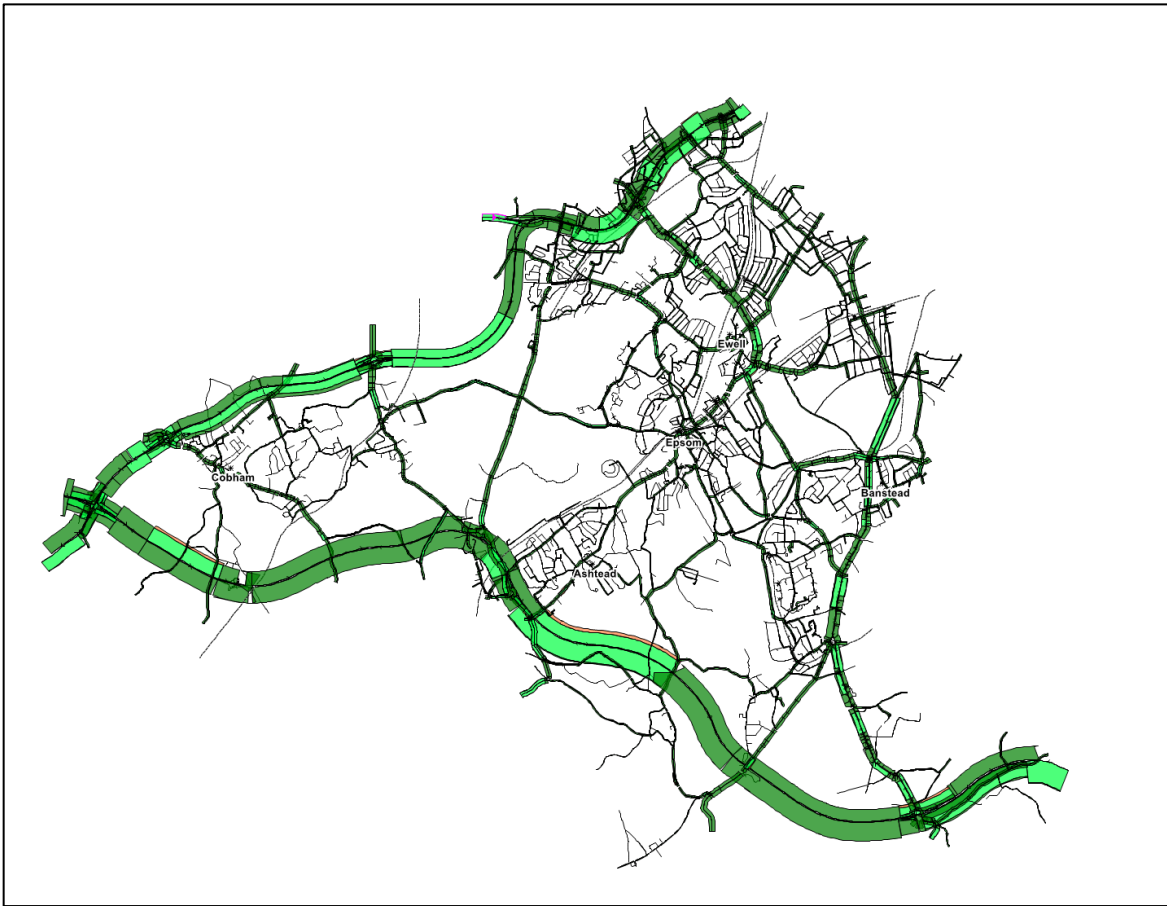
Figure 27 Local Model Link Flow versus Count Bandwidth for the AM Peak Hour (0800 – 0900) with all roads showing above and a close up of Epsom and Ewell below
