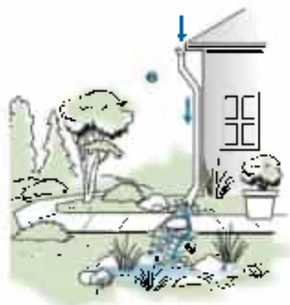
Disconnected drainpipe discharging into a small pond ( http://www.portlandonline.com )
